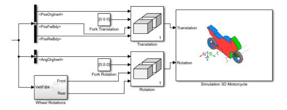
Previously, the Motorcycle Body Longitudinal In-Plane block did not contain signals to easily provide the Simulation 3D Motorcycle with the motorcycle motion.
